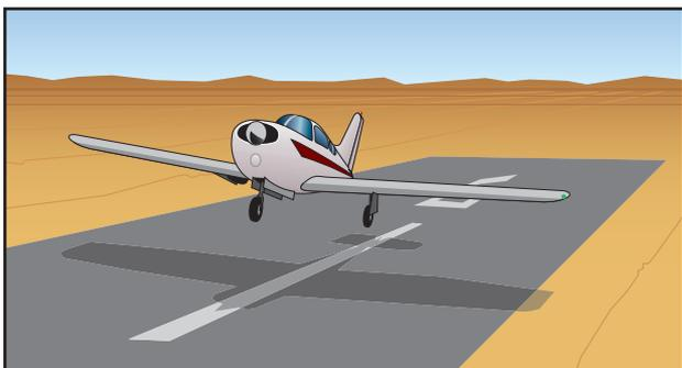
Figure 16-7. Landing with one main gear retracted.
